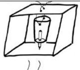
**8** With the string, suspend the cup from the holes in the box so that the tip of the pen touches the bottom of the box.
